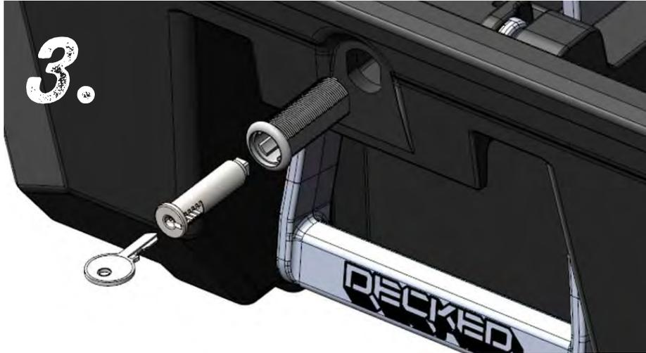
**STEP 4:** WITH LOCK CORE INSERTED AND SQUARE TAB ON LOCK BARREL AT 12 O'CLOCK, SLIDE GOOFY SHAPED WASHER ONTO LOCK CORE SUCH THAT THE STOPS ON THE WASHER ARE AT 9 O'CLOCK AND 12 O'CLOCK. THE 12 O'CLOCK STOP ON THE WASHER SHOULD BE POSITIONED AS SHOWN IN DIAGRAM 4.
