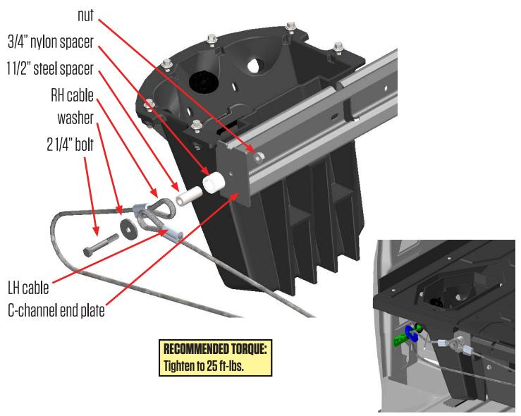
Enlargement of RH cable assembly attachment to connecting link (blue).
